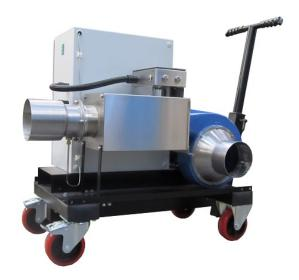
The industrial fan and process heater are mounted to a base frame including hose connectors for the outlet (and inlet on recirculating systems). Braked castors and an adjustable height handle can be fitted if required to produce a Mobile Heat Pack unit. All or part of the element load is switched using solid state relays to give accurate temperature control. Start and stop buttons are provided and also prevent the heater being operated without the fan.
